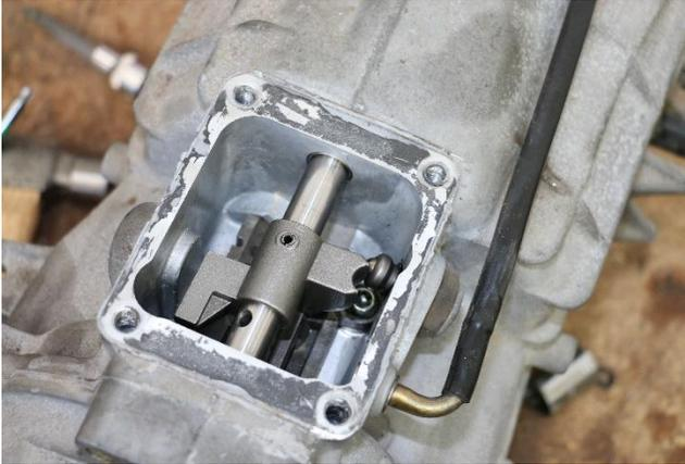
in this set up it can be retained and will make selecting neutral easier. The easiest way to check is to rotate the shaft fitting while in neutral, if it stays to the side with minimal force ( 1<sup>st</sup> or 5<sup>th</sup> side of the gate you have the t56 style if it has a strong return to centre force you have the Magnum/Tr6060 style.
